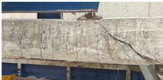
Fig. 7 Crack pattern of Beam BS01
